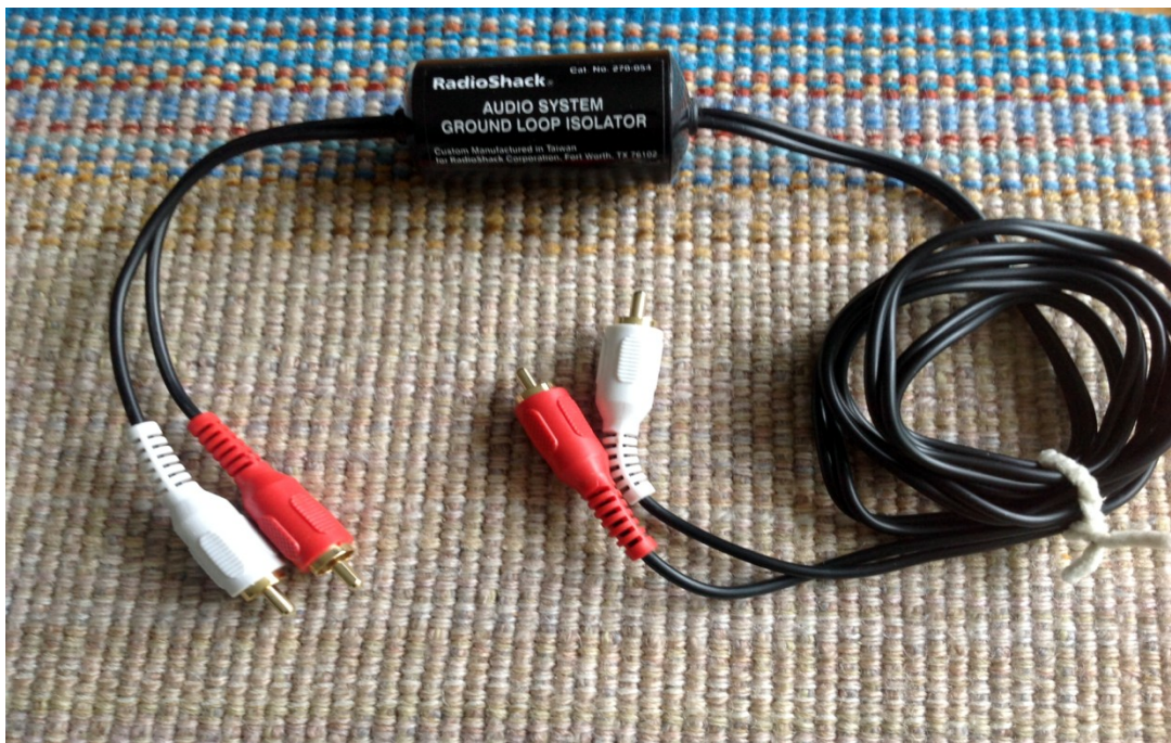
Shielded audio cables with a 1:1 isolation transformer
